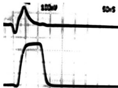
Figure 12: SJ Monitor Test: 150 \Omega Fault Causes an I/O Pin Perturbation (Top) That is Detected (Bottom); Fault Duration Was About 50ns - X-axis is 50ns and Y-axis is 100mV.
