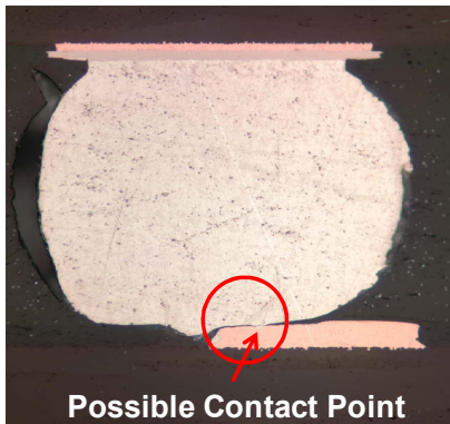
Figure 21. Fault not detected: board 6, FPGA 3, pin A24.
