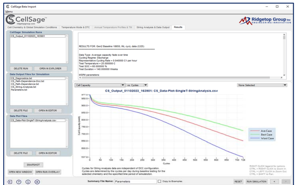
Example of Path Dependent Capacity Loss for best-case, average-case, and worst-case scenario in CellSage™ GUI
