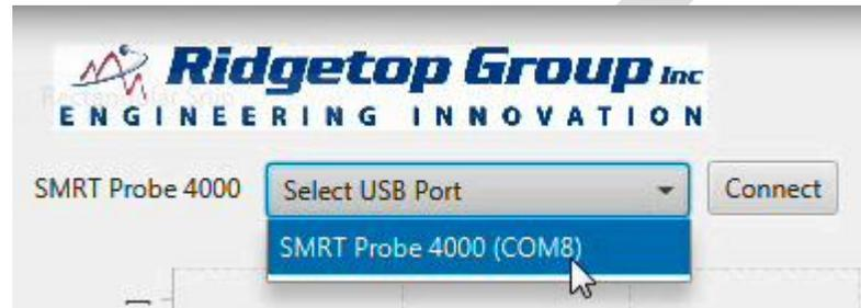
Figure 9: Selecting the correct COM port
