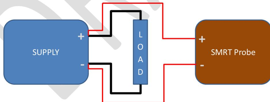
Figure 5: SMRT Probe 4000 application diagram
