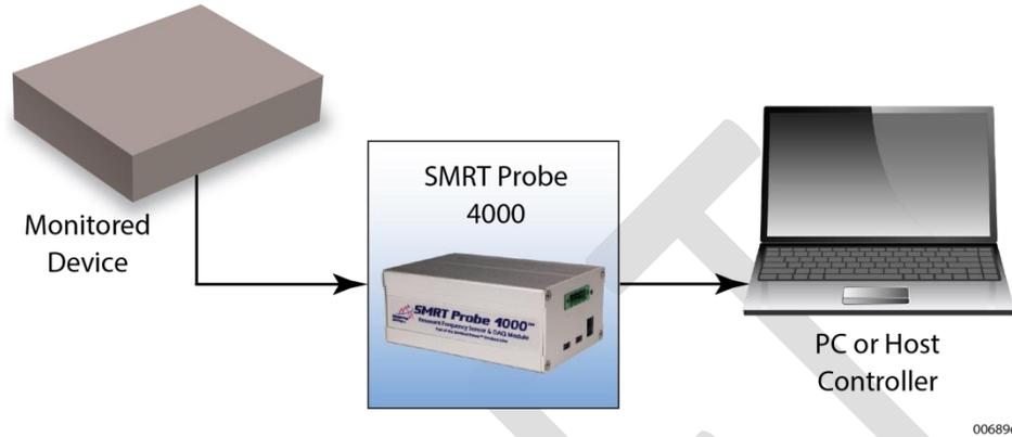
Figure 2: System diagram of SMRT Probe 4000 operation
