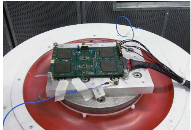
Figure 20: HALT Test Board Mounted on Vibrator.
