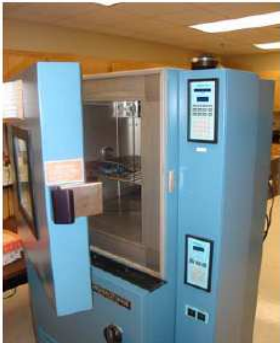
Figure 19: Thermal Oven for Solder Joint HALT Testing – CAVE, Auburn University, Alabama.
