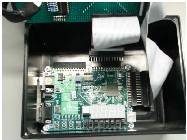
Figure 19: SJ BIST Demonstration Box, XILINX Spartan 3 Board.
