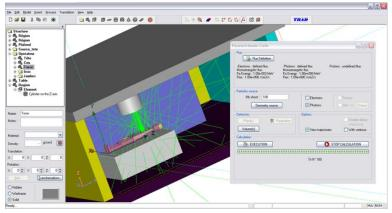
RadChek is a tool that rapidly computes the radiation effects on electronic boards and modules destined for harsh environments where radiation is found, such as in space, or near equipment such as particle accelerators, nuclear power plants, or medical scanners. RadChek's analysis capability allows engineers to determine the best shielding material to use to avoid the damaging effects of radiation.
