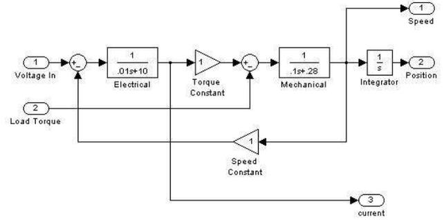
Figure 10: DC Motor (Simulink Model)
