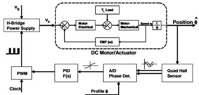
Figure 7: State Diagram of a Close-Loop DC Motor/Actuator System
