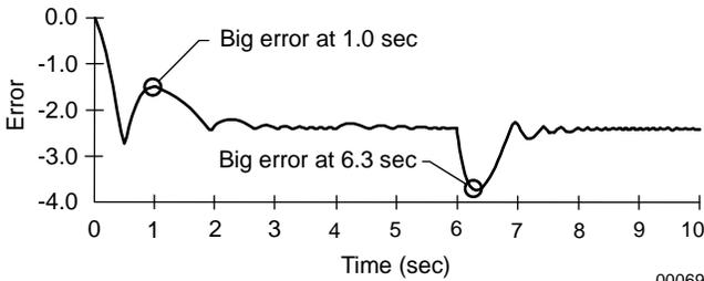
Figure 17: Simulated Following Error (M1 or M3 are damaged) (Simulink Model) 00069
