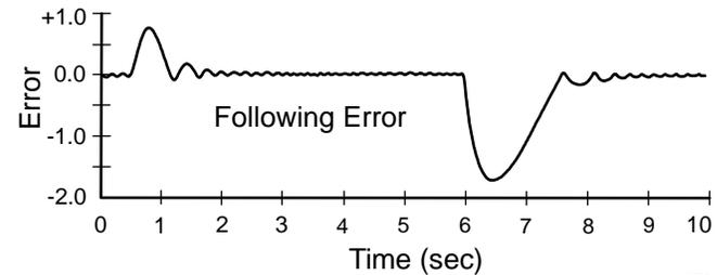
Figure 15. Simulated Following Error (All MOSFETs are good) (Simulink Model)
