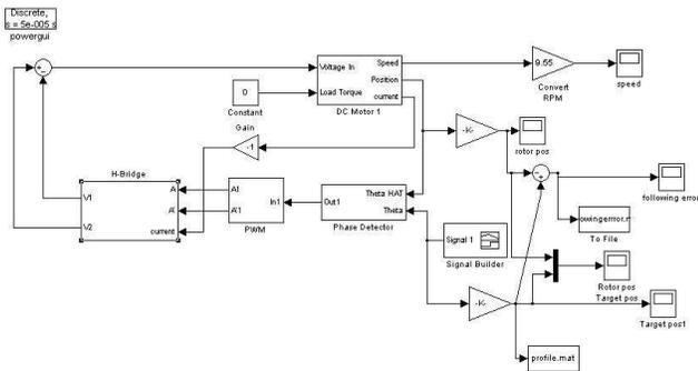
Figure 9: Actuator Circuit (Simulink Model)
