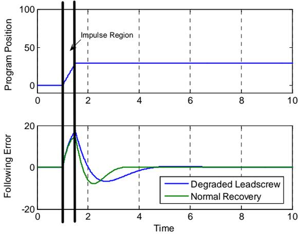
Figure 8: An Impulse Response in an Actuator Caused by a Position Jog
