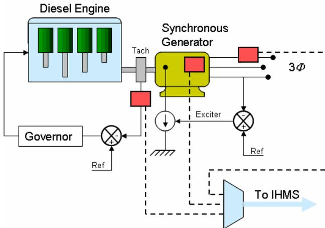
Figure 20: A System-Level Solution for Synchronous Generator
