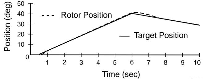
Figure 14: Simulated Target Position vs. Rotor Position (All MOSFETs are good) (Simulink Model)
