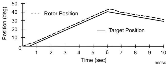
Figure 16: Simulated Target Position vs. Rotor Position (M1 or M3 are damaged) (Simulink Model) 00066
