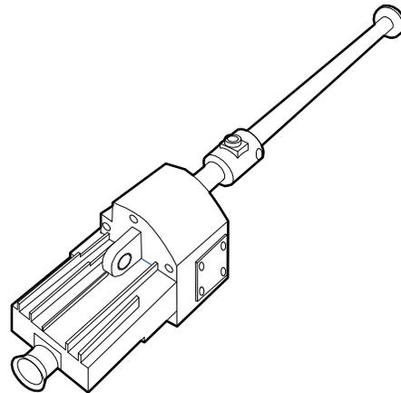
Figure 1: A Linear Actuator
