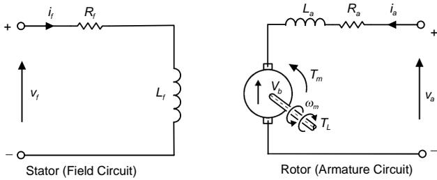
Figure 11: Equivalent Circuit of a DC Motor and Armature Mechanical Loading Arm
