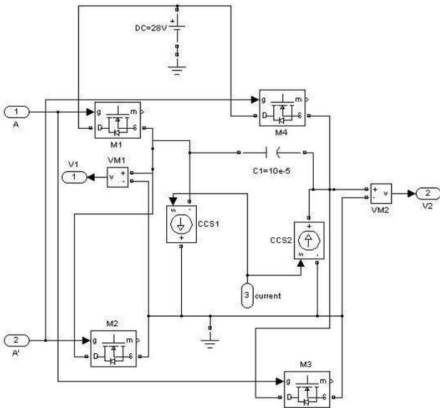
Figure 13: H – Bridge (Simulink Model)
