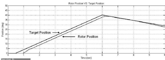
Figure 18: Simulated Target position vs. Rotor position (M2 or M4 are damaged) (Simulink Model)
