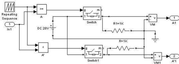
Figure 12: PWM Circuit (Simulink Model)
