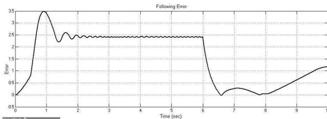
Figure 19: Simulated Following Error (M2 or M4 are damaged) (Simulink Model)
